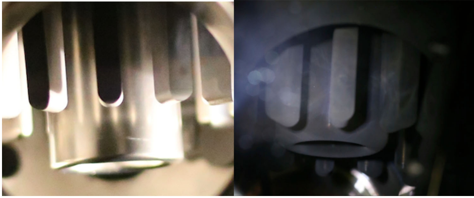
Fig. 8 Our 2021 polished beryllium anode (left) still shined mirror-bright after three shots in August, 2021. It is viewed through a window on our vacuum chamber. The anode is a bit more than 5 cm in diameter. The colors on the anode seen here are the result of lighting and camera response. The true color of the anode is still
