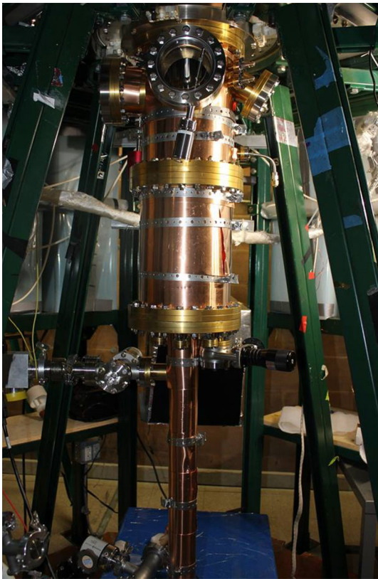
Fig. 5 Vacuum chamber and drift tube of FF-2B
