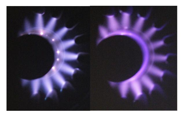
We started in July (left) with a very unsymmetric breakdown, with the current focused in the bright spots. Now (right) the breakdown is more symmetric, with the current mostly spread out in the pink ring and just a little in the two bright spots. The anode (central black region) looks oval in the right-hand image because the current is concentrated in a thin sheath while in the left-hand image, it spreads out up the side of the anode. Change in color is due to the addition of a mixing gas.
