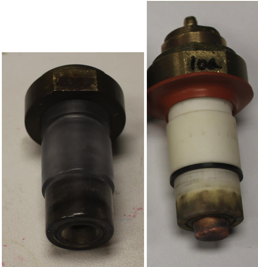
Figure 3. The darkening of the Lexan insulators (left) led the LPPFusion team to replace them with ceramic ones (right). However, the ceramics were much more prone to surface breakdowns within the switch, as evidenced by the dark stripes on the bottom of insulator, near the copper center pin. They also had breakdowns outside the switch, as evidenced by the thin dark marks on top and in the middle of the insulator, which the red rubber guard also failed to stop. We now have a more effective guard at the top of the insulator. Teflon is better at resisting surface breakdown than either Lexan or the aluminum oxide ceramic, so will be tried next.
