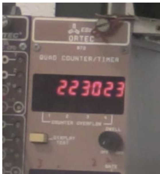
Figure 2. LPPFusion's silver activation counter shows 220 billion neutrons, or about 1/4 of a joule of fusion energy, from cleaning shot 1, March 27 with deuterium fuel. This matches, within 10%, our record fusion yield.
